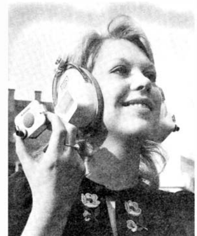
This ear defender headset permits a wearer to work in noisy environments without discomfort while still being able to hear normal speech. The earphone providing the signal to the wearer is in the inner shell of the set while the amplifier components are in a clip-in module (held by the girl in the picture). A controlled-sound transmission channel cuts out any noise above 85dB
